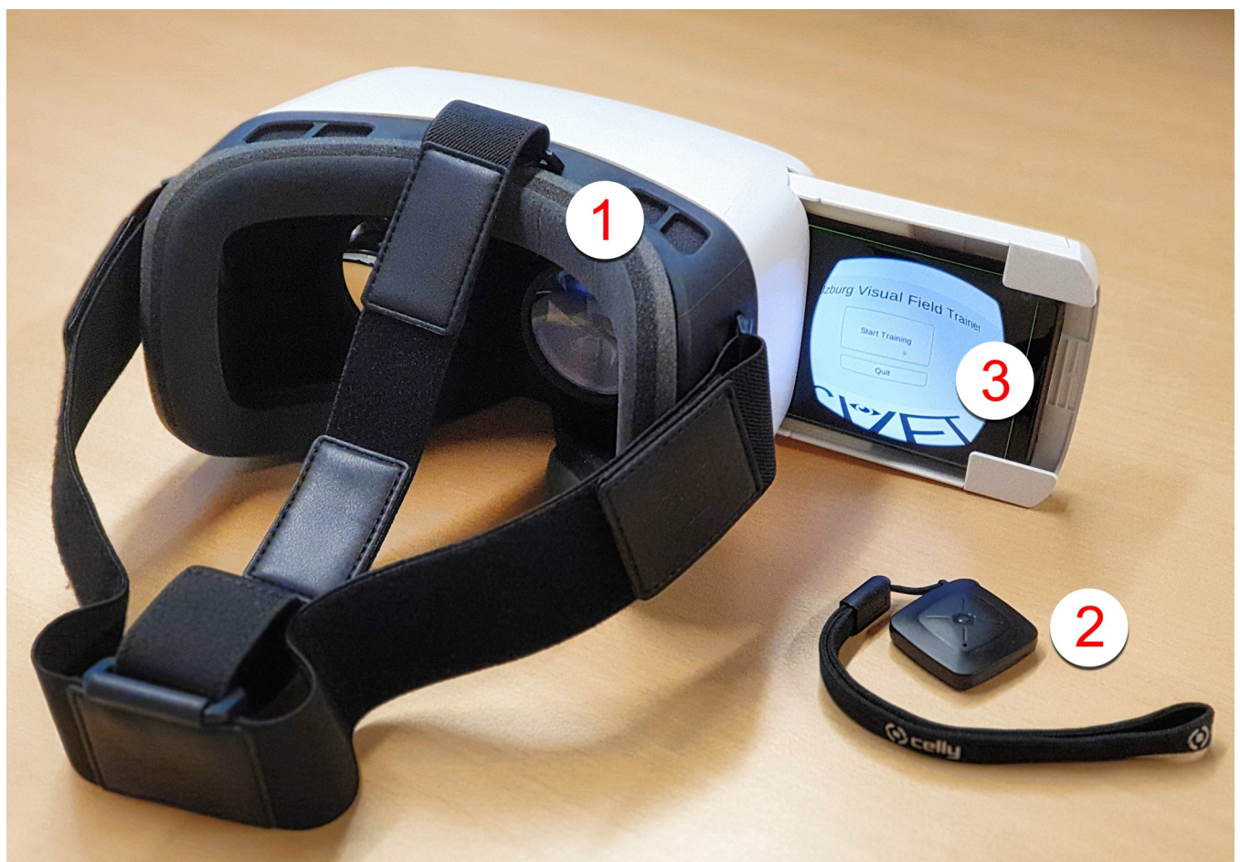
Fig 2. Setup of the “Salzburg Visual Field Trainer” (SVFT). Figure illustrates Google® Cardboard based solution (1) ZEISS® VR ONE Plus, (2) Celly® Bluetooth® remote control and (3) Samsung Galaxy S9® smartphone (SM-G960F/DS). The smartphone runs software coded in Unity® on Android® Pie operating system. By clicking on the Bluetooth® remote control during training, the user gives feedback to the system, which enables main menu navigation and adapts the position of the presented stimulus during the course of training. Thus, the presented stimuli keep being displayed in the individual transition zone of the user’s intact and defect visual field after potential improvements stemming from neuronal reconnection.
