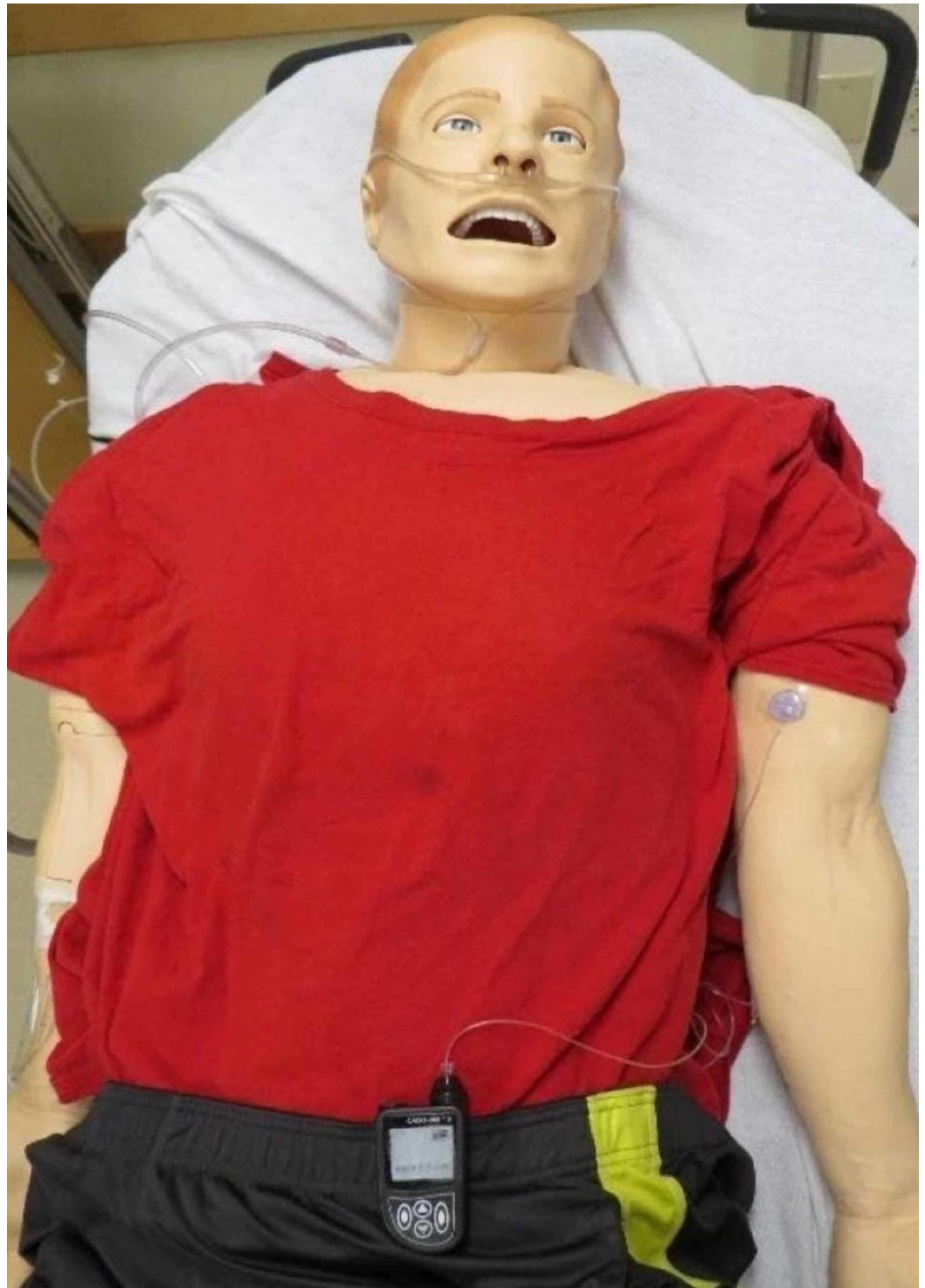
FIGURE 4: Subcutaneous Remodulin® pump mannequin setup
