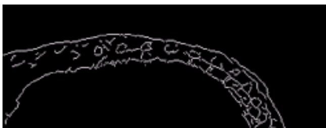
Figure 3 Edge Detected Image. This is the result of Canny edge detection when the image has not been segmented. Note that most of the edges required are missing from this image.
