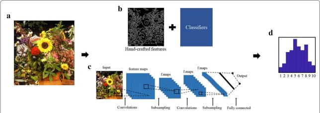
**Fig. 3** A workflow for image quality assessment. **a** The original image. **b** Hand-crafted features are extracted by computational algorithms and subsequently feed to classical classifiers. **c** Using neural network to automatically extract image features related to aesthetic ratings. **d** Final prediction
