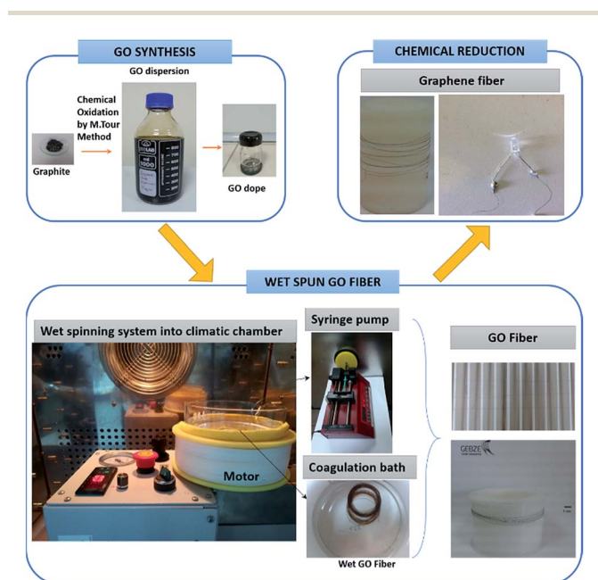
Fig. 1 Wet-spinning system to obtain GOFs and GF filament from graphite.
