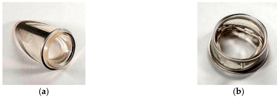
Figure 9. Polymer components of the valve rings: (a) the inflow and (b) outflow valve.
