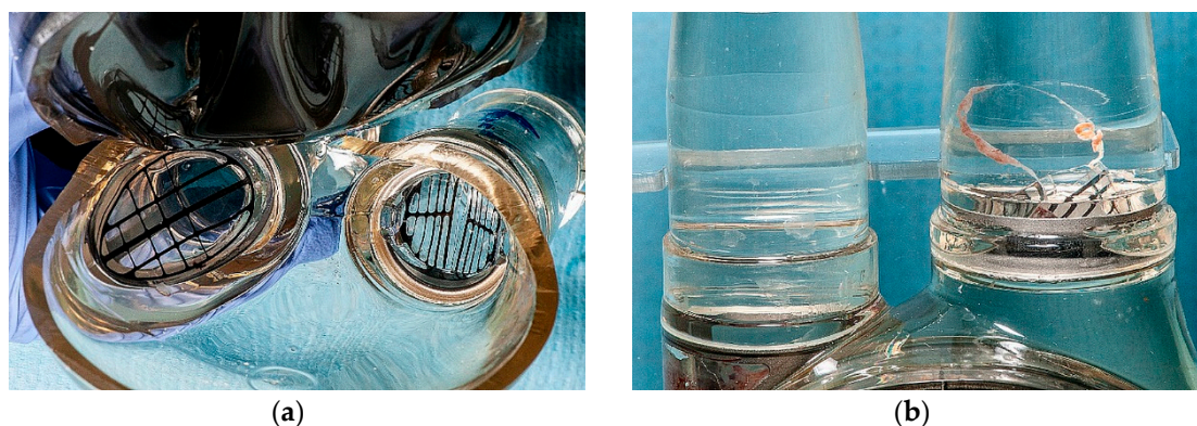
Figure 19. View of valves after in-vitro thrombogenicity study: (a) view from the inside of the blood chamber on the inflow and outflow valves, (b) side view at the place where the valves are glued in.
