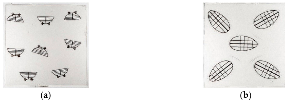
Figure 10. Foils with stiffening frames made of titanium after pressure processing for (a) outflow and (b) inflow valves, respectively.
