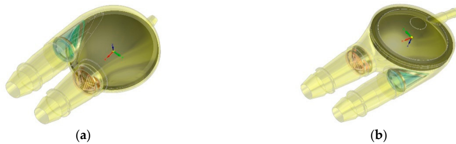
Figure 6. ReligaHeart EXT heart assist pump with new valves (a) view from the side of the blood chamber, (b) view from the pneumatic chamber.
