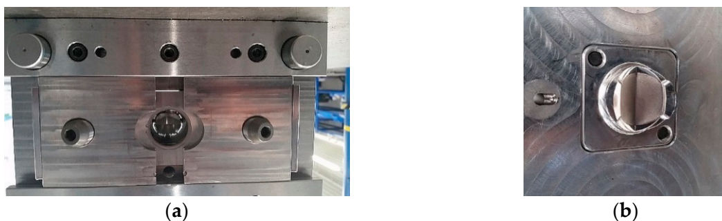
Figure 8. Injection mold for the ring of the outflow valve: (a) mold seat and (b) mold stamp.
