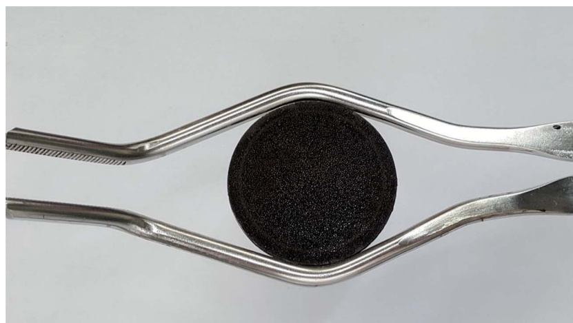
Fig. 6 Carbon membrane prepared using dip-coating with 3 : 1 concentration.
