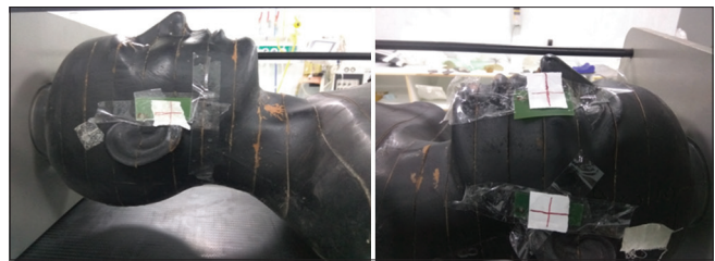
Figure 6: In vitro verification of dose difference to the skin by skin spared IMRT using Gafchromic film dosimetry, IMRT: Intensity modulated radiation therapy
