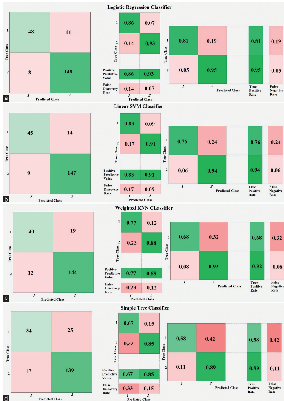
Figure 3: Two-class classification confusion matrices using 10-fold cross-validation for (a) logistic regression, (b) linear support vector machine, (c) weighted K-nearest neighbor, and (d) simple tree classifiers
