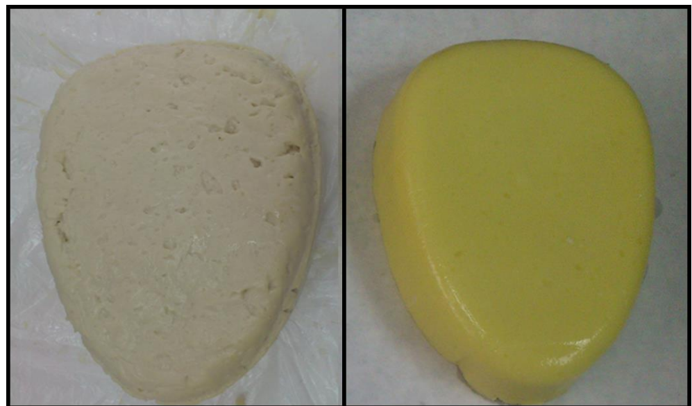
Figure 3. Representative appearance of oil-free SPI gel (SPI/G, left) and SPI emulsion gel (SPI/EG, right). For sample denomination see Table 1.
