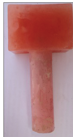
Figure 1: The acrylic cylinder fixed to the bottom of the acrylic base block
