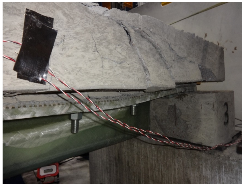
Figure 15. Post-Failure Image of Beam B1.
