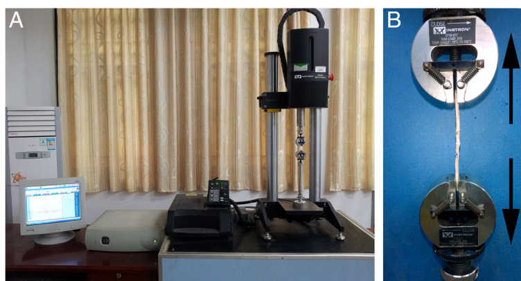
Figure 1 The Instron Model 5848 MicroTester (A) and specimen attached to the tester (B).
