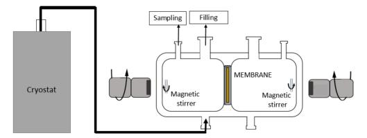
Figure 3. The scheme of the pertraction setup [48].
