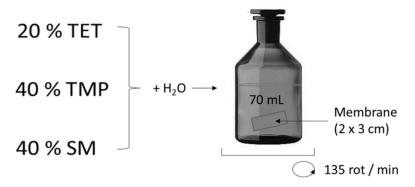
**Figure 2.** The membrane sorption of the antibiotics—tetracycline (TET), sulfamethoxazole (SM), and trimethoprim (TMP).
