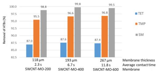
Figure 12. Rate of removal of ATBs for different membrane thicknesses versus average contact time.
