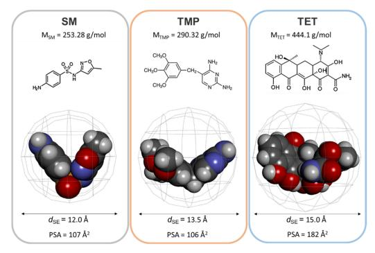
**Figure 10.** A comparison of the molecular weight ( $M_{ATB}$  in g/mol), structural formula, diameter of the spherical enclosure ( $d_{SE}$  in Å), and polar surface area (PSA in Å<sup>2</sup>) for SM, TMP, and TET.
