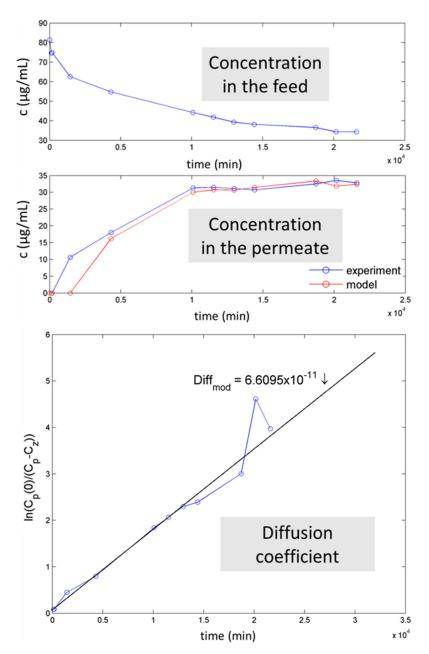
**Figure 14.** Concentration in the feed and permeate in time and an example of the calculation of the diffusion coefficient.
