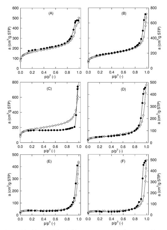
**Figure 6.** Adsorption ( $\bigcirc$ ) and desorption ( $\bullet$ ) branch of the nitrogen sorption isotherm for SWCNT-200 (**A**), SWCNT-200 (**X**), SiO<sub>2</sub> (**B**), SWCNT-200  $\nearrow$  SiO<sub>2</sub> (**C**), Mod\_SWCNT-200 (**D**), Mod\_SWCNT-200 (**X**), SiO<sub>2</sub> (**E**), and Mod\_SWCNT-200 (**X**), SiO<sub>2</sub> (**F**).
