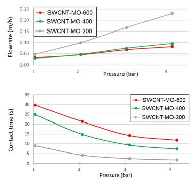
**Figure 11.** Flow rate and contact time of SWCNT-MO-200, SWCNT-MO-400, and SWCNT-MO-600 membranes as a function of the pressure.
