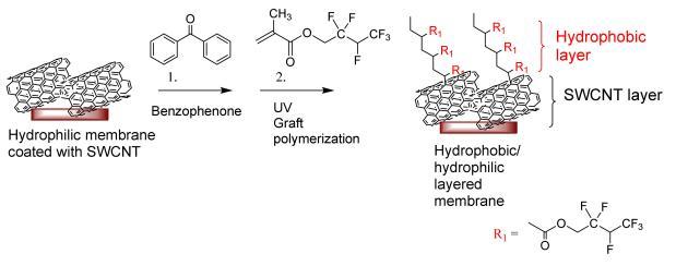
Figure 1. The graft-polymerization results in a hydrophobic layer on top of the SWCNT layer.
