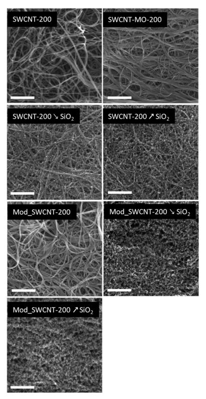
Figure 4. SEM images of the membrane surfaces. Scale bar corresponds to 500 nm.
