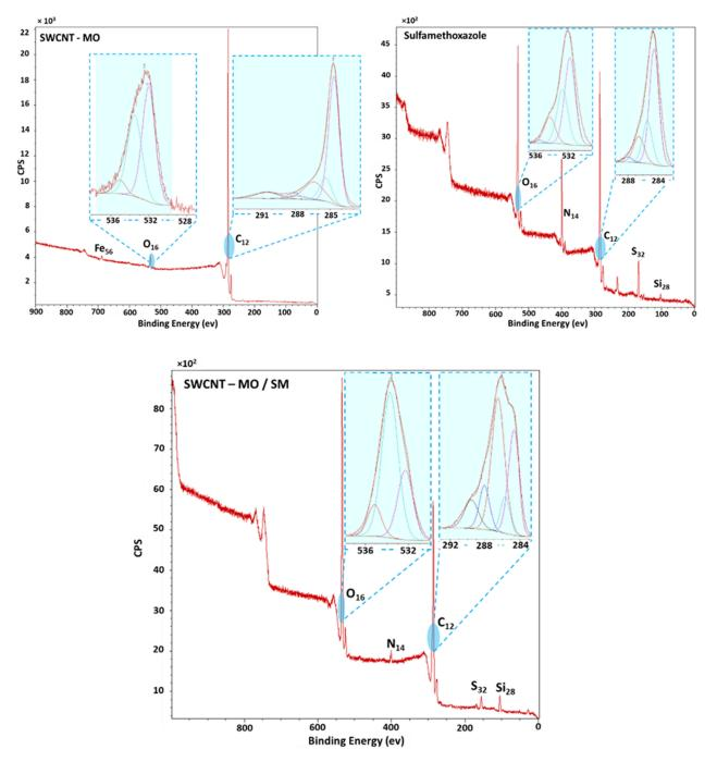
Figure 16. XPS spectra of the fresh and the used membrane SWCNT-MO-200 for SM sorption.
