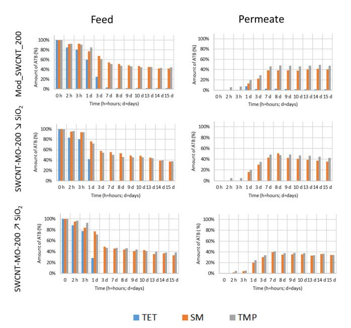
Figure 13. The amount of ATBs (%) in the feed and in the permeate for the modified membranes as a function of time.
