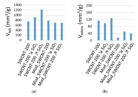
Figure 5. (a) Total pore volume; (b) micropore volume, determined from the N<sub>2</sub> adsorption isotherms.
