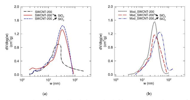
**Figure 7.** Pore size distribution evaluated from the desorption branch of the nitrogen sorption isotherm at 77 K: for unmodified (**a**) and modified (**b**) membranes by a hydrophobic layer.
