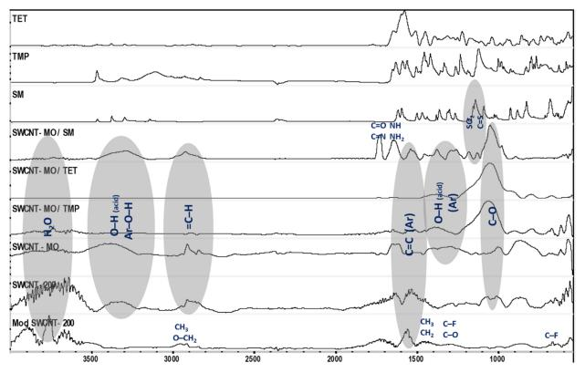
Figure 15. FTIR spectra of TET, TMP, SM, and selected membranes.
