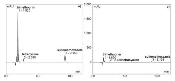
**Figure 8.** HPLC spectra of a mixture of ATB at time zero (**a**), a mixture of ATB after 1 day (**b**), and the SWCNT-MO-200 membrane.
