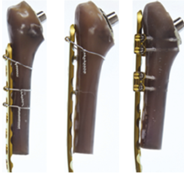
FIGURE 2: Humerus-LCP construct after performing the transverse osteotomy 5 cm distal to the end of the prosthesis, with the irreversibly bent LCP after performing the biomechanical stability testing.
