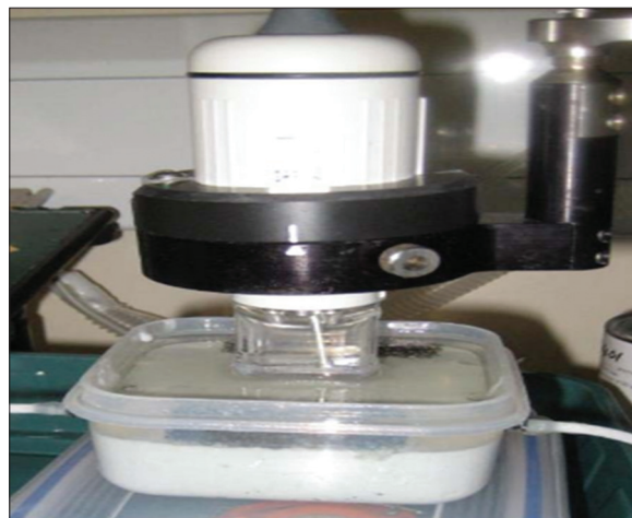
Figure 4: Konjac carrageenan-based tissue-mimicking material flow phantom used with the Visualsonics Vevo 770 preclinical scanner [14]
