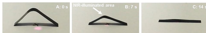
Figure 12. The shape recovery of V-fa/ECO SMPCs filled with MWCNT using NIR laser irradiation (adapted from [47]).
