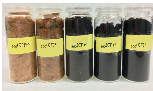
Figure 1. Pictures of the CFs synthesized at 300 °C.
