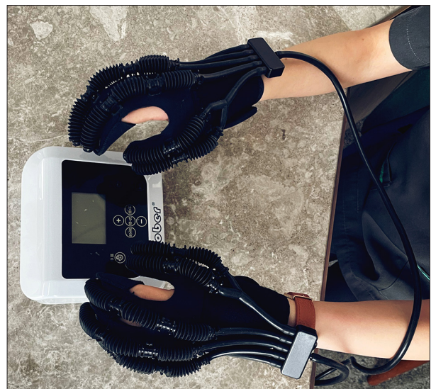
Figure 8. Hand strength rehabilitation demonstration. The patient is wearing robotic gloves (Ober, China) and conducts fine motor activities for up to 30 min per day. Also shown is the control console that allows the level of mechanical assistance to be altered. Image from EC.
