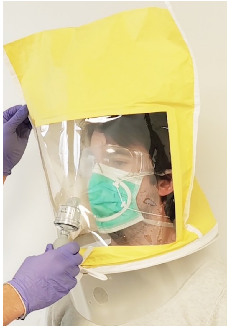
Fig 3. An individual of the intervention group being submitted to the qualitative fit test with the hood and nebulizer of the 3M FT-10 fit test.
