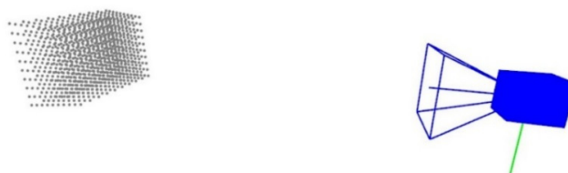
Figure 8. A virtual pyramid for camera calibration with 1000 points ( 10 \times 10 \times 10 ), which is displayed in an internal software to obtain intrinsic and extrinsic parameters.
