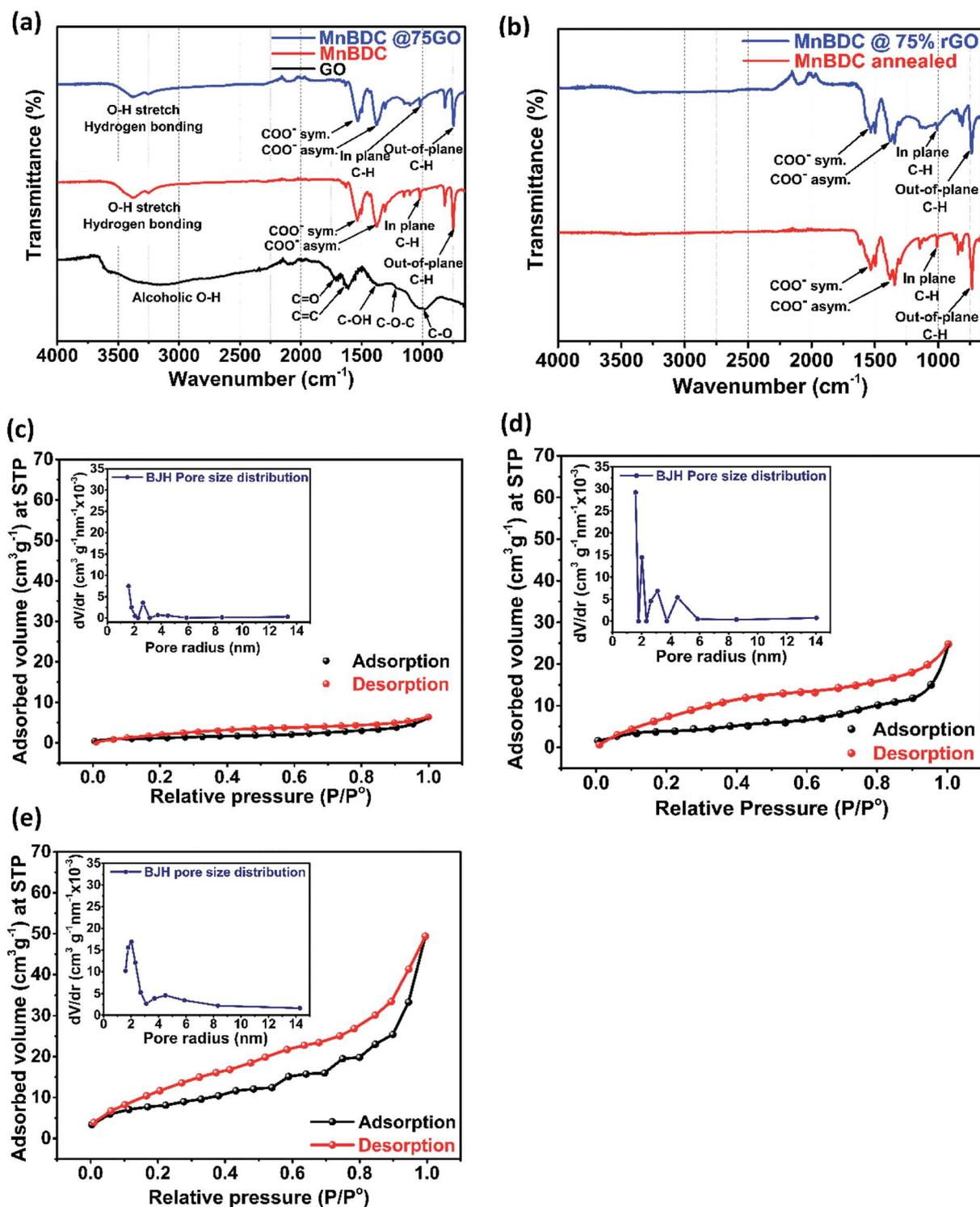
Fig. 2 FTIR spectra of (a) GO (black), MnBDC (red), MnBDC@75% GO (blue), (b) post annealing samples of MnBDC (red) and MnBDC@75% rGO (blue). N<sub>2</sub> sorption isotherm along with BJH pore size distribution profile as inset of (c) MnBDC, (d) MnBDC@75% GO and (e) MnBDC@75% rGO.
