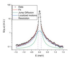
**Figure 6.** Fit example of Tba PMI at 1 bar and 286 K, at a q value of 1.14 Å $^{-1}$ . Black circles represent the corrected data, the two Lorentzian contributions owing to localized motions and jump–diffusion are shown respectively as blue and green solid lines, and the total fit is shown as a red solid line. The resolution function is also shown. Error bars are smaller than the symbol size.
