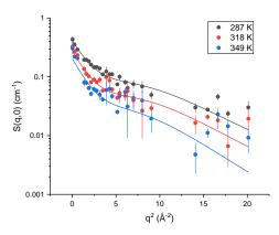
**Figure 3.** Scattering curves for Tba PMI at 150 bar and at some representative temperatures, with the corresponding two-state model fits. The decrease of the elastic intensity with temperature is expected, as more motions enter the time window of the experiment and the involved atoms scatter neutrons inelastically.
