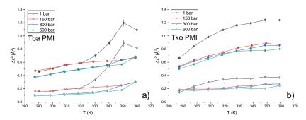
**Figure 4.** Total MSD (full circles) and MSD into the single wells ( $\Delta x_0^2$ , open circles) for Tba PMI (**a**) and Tko PMI (**b**), lines are a guide to the eye. The absolute value of the MSD reports on the amplitude of hydrogen atoms motion, while the slope of the curve as a function of temperature indicates how much energy is necessary to increase said amplitude, i.e., the *resilience* of the protein [32].
