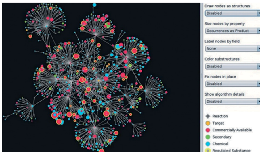
Fig. 4 Complex tree-search network in Chematica. Nodes can be displayed as 2D or 3D molecular structures (for basic modelling calculations) and can be expanded down the retrosynthetic path. Blue nodes denote products; green are minor/side-products, red are commercially available substances, and yellow halos denote regulated substances. Reproduced from ref. 53.
