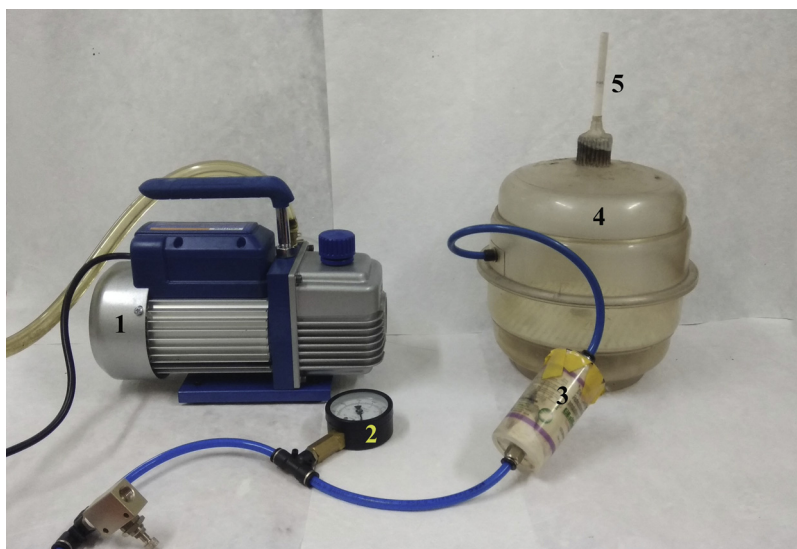
Fig. 1. The smoker chamber used to expose guinea pigs to cigarette smoke. 1. The vacuum pump, 2. Pressure gauge, 3. Filter (to trap tar), 4. The vacuum desiccator that acts as the smoke chamber, 5. Cigarette holder containing the cigarette.
