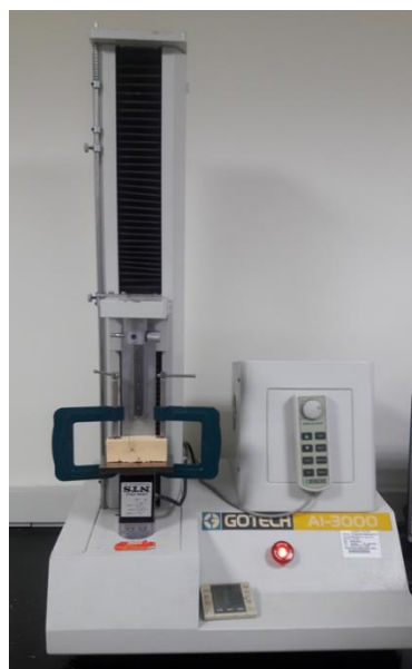
Figure 6. An orthodontic wire (0.018 inch) was passed through the hole of microimplant, then tied into the material testing machine (GOTECH AI-3000, Gotech Testing Machines Inc., Taichung, Taiwan).
