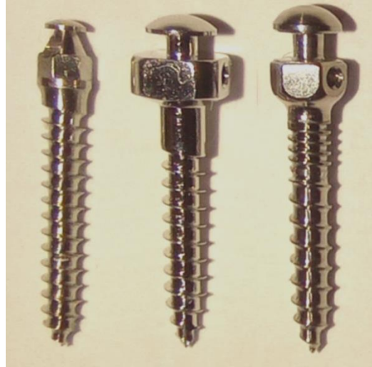
Figure 1. Microimplants manufactured with 3 designed types, from left to right: Type A. 5 \times 10 mm; no microthread neck), Type B ( 1.5 \times 10 mm; no microthread neck), and Type C ( 1.5 \times 10 mm; microthread neck).
