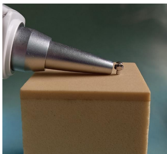
Figure 5. Tapping head device of the Periotest system (Periotest M, Medzintechnik Gulden, Modautal, Germany) to percuss the microimplant.
