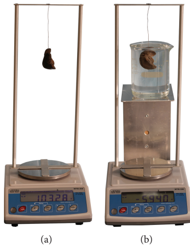
FIGURE 1: A double weighing procedure to obtain the weight of the liver in air (a) and distillate water (b).
