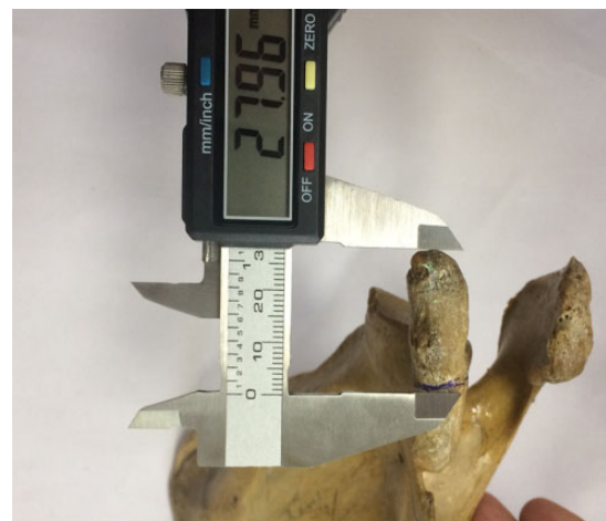
Figure 7. Length measurement with handheld calipers.
