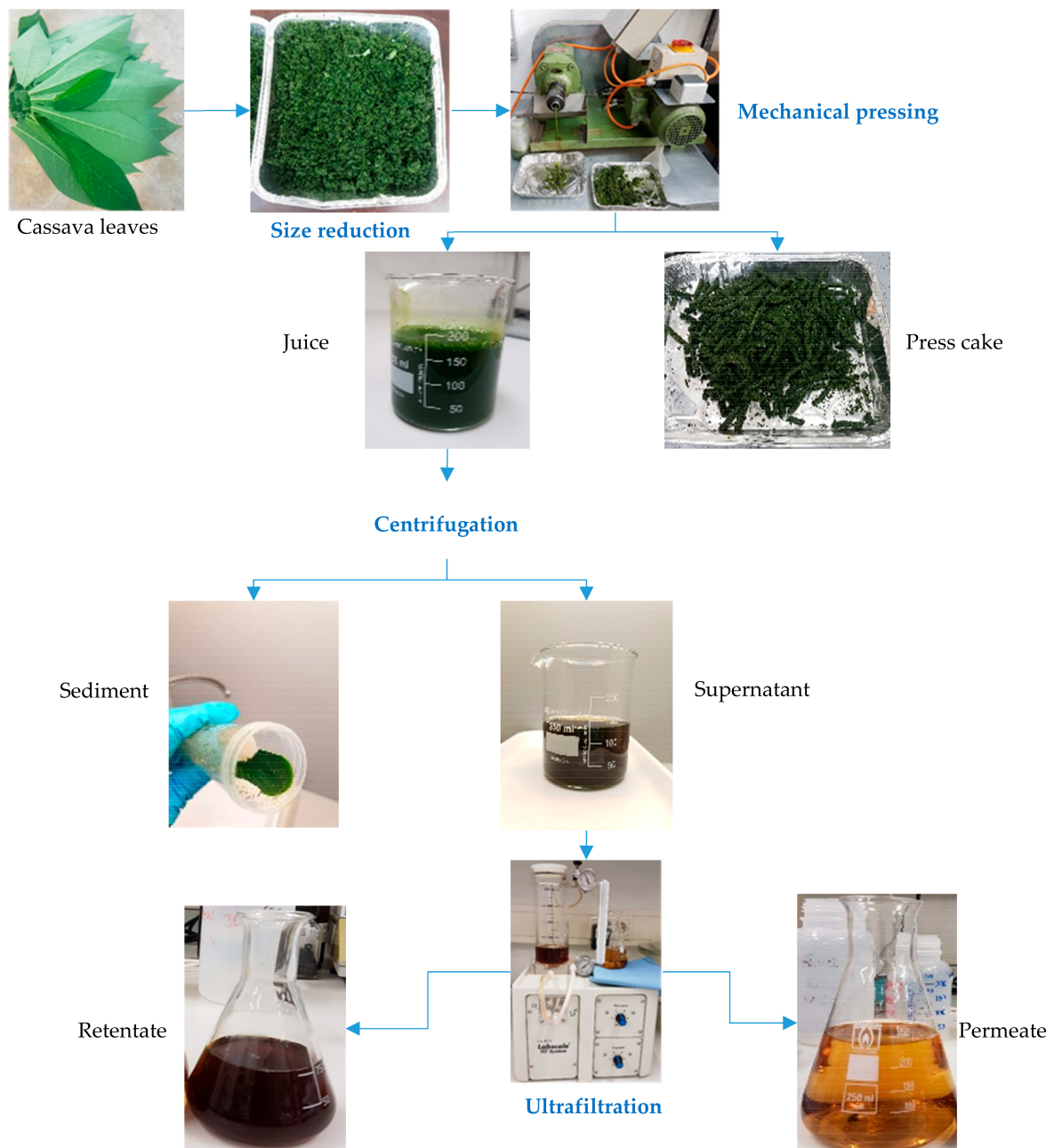
Figure 1. Cassava leaf processing via mechanical pressing and ultrafiltration.
