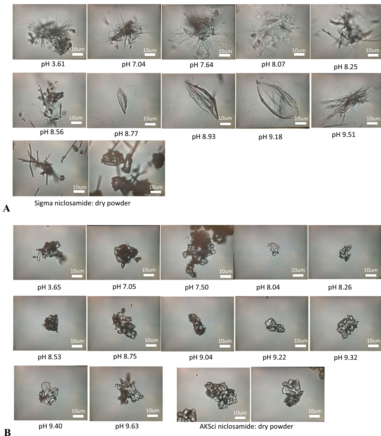
Fig. 14 A Optical microscope images of excess Sigma Niclosamide powder particles after overnight equilibration over the whole pH range from 3.61 to 9.51. This overnight equilibration produced long rod-like, needle-shaped, and spiky-bundled structures at all pHs tested showing that the Sigma niclosamide converted to the lower solubility polymorph as the lower solubility monohydrate. These hydrated samples are compared to the dry, as-received, powder from the Sigma supplier that already showed a considerable amount of rod like and needle-shaped crystal morphology in addition to a more block-like morphology. B . Optical microscope images of excess AKSci Niclosamide powder particles after overnight equilibration over the whole pH range from 3.65 to 9.63. In contrast to the Sigma niclosamide samples, this AKSci material retained its original block-like morphology at all pHs tested. There was a distinct absence of the prototypical spiky bundled morphology characteristic of the monohydrate. Thus, the AKSci material did not convert to the lower solubility needle-shaped monohydrate. These hydrated samples are also compared to the dry, as-received, powder from the AKSci supplier that have the block-like morphology.
