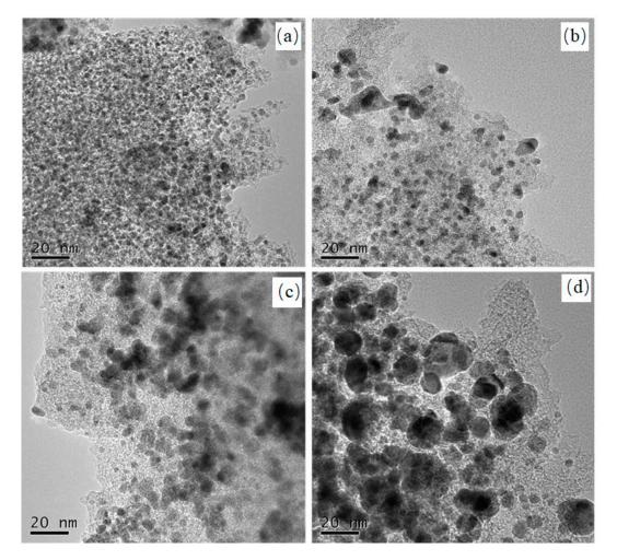
**Figure 6.** TEM images of the Pd/C catalysts fresh (**a**), after 6 cycles of hydrogenation in water (**b**), after 6 cycles of hydrogenation in ethanol-water (50/50) (**c**), after 6 cycles of hydrogenation in ethanol (**d**).
