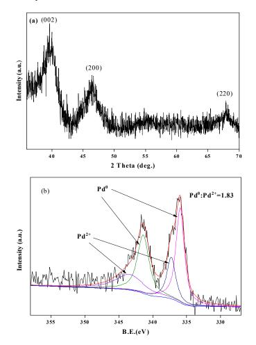
Figure 2. (a) XRD and (b) X-ray photoelectron spectroscopy (XPS) patterns of Pd/C.
