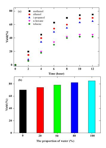
**Figure 4.** Hydrogenation of naringin in different solvents over 10 wt % Pd/C catalyst. (**a**) Hydrogenation of naringin in various solvents. (**b**) Hydrogenation of naringin in various ethanol–water mixtures. Reaction conditions: 150 mL of each solvent, 5 g of naringin, solvent pH 12, 0.5 g of 10 wt % Pd/C(0), temperature of 45 °C, and H<sub>2</sub> pressure of 1.5 MPa.
