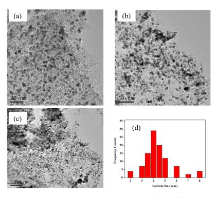
**Figure 1.** Transmission electron microscopy (TEM) images of 10 wt % Pd/C with different magnifications (**a**–**c**) and size distribution of Pd particles (**d**).
