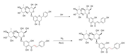
Scheme 1. The reaction scheme of hydrogenation of naringin.
