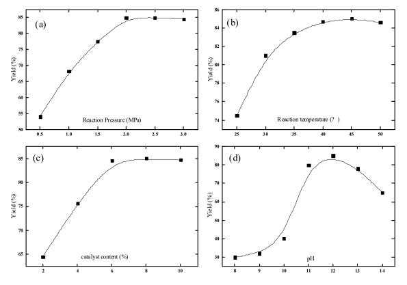
**Figure 7.** Effects of reaction pressure (**a**), temperature (**b**), catalyst content (**c**), and pH (**d**) on the DHC yield. The Reaction conditions: 150 mL of each solvent, 5 g of naringin, solvent pH 12, 0.5 g of 10 wt % Pd/C(0), temperature of 45 °C, and H<sub>2</sub> pressure of 1.5 MPa.
