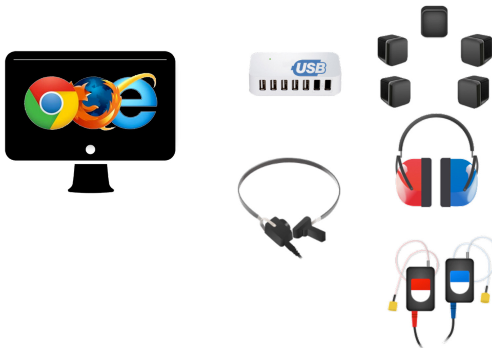
Fig. 2. Principle of digital audiometry with air and bone conduction stimulation (headphones, earphones, free field). Any connected computer can be use as an audiometer, the transducers being connected to a USB port, for example. Resources are thus centralised: multilingual word lists, test protocols and results, questionnaires, creation of audiological databases.
