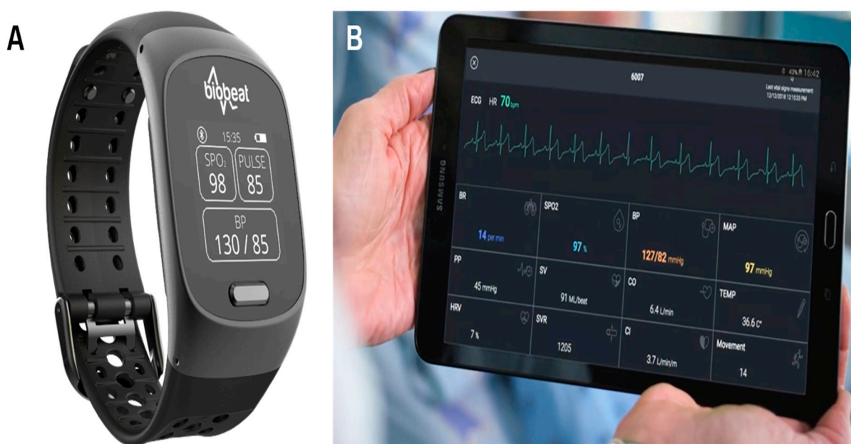
Figure 1. The Biobeat remote patient monitoring platform. (A)The wristwatch device. (B)Real-time measurement collected by the device.
