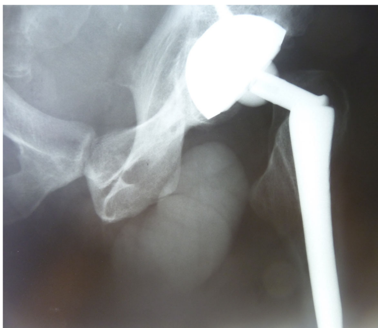
Fig. 1 Emergency room X-ray of the left hip with fractured modular femoral neck 3 years after primary THA
