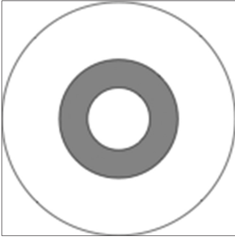
Figure 1: Schematic design of refractive intraocular lenses showing the different refractive power annular zones
