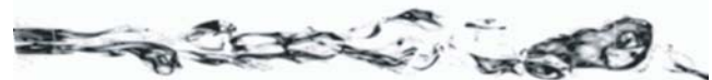
Figure 2. Visualization of a pheromone plume. The figure is extracted and adapted from a digitized image of a smoke plume filmed in a wind tunnel 1 m across and 2 m long with source on the left side [43]. Though the average pheromone concentration in the air decreases with distance, high pheromone concentrations can be found relatively far from the source due to the imperfect mixing of odorant with air. The signal detected by both moving and stationary detectors is therefore always intermittent, consisting of pulses of relatively undiluted pheromone. doi:10.1371/journal.pcbi.1000053.g002
