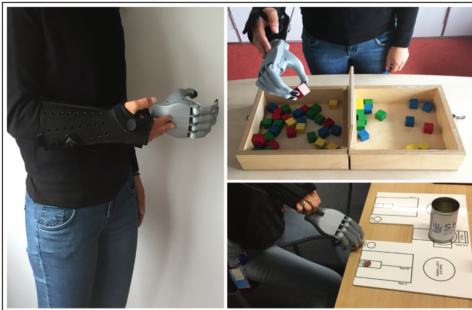
Figure 5. Our 3D-printed prosthetic hand attached to the simulator and used by the participating subjects (left) for the Box and Blocks test (top right) and the SHAP test (bottom right). Gaffer tape strips were put over the thumb, the index, and middle fingers to increase grip (right).
