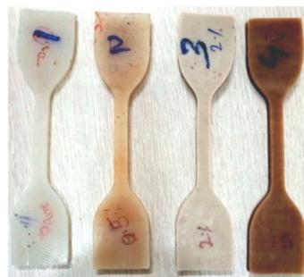
Figure 2. Samples prepared for tensile testing.
