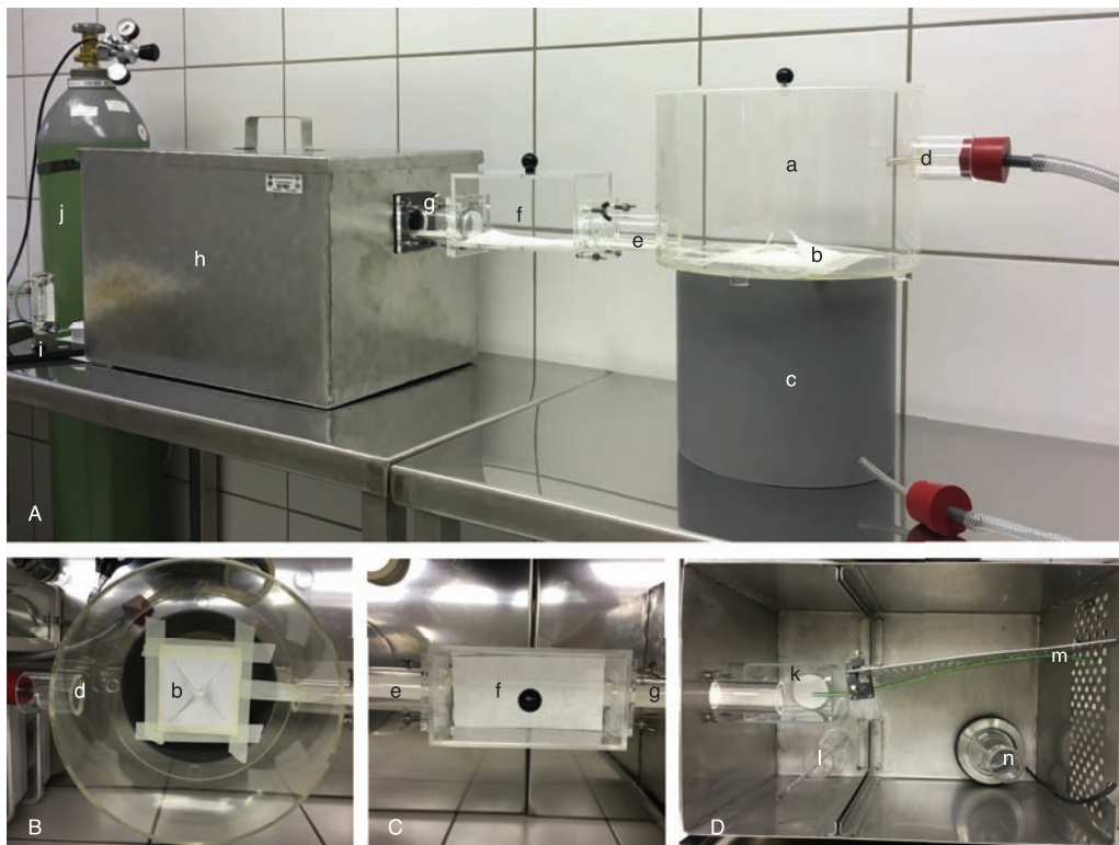
Fig. 2. Barrier test system. (A) Overview of the test setup; (a) cylindrical container; (b) kitchen paper towel pocket; (c) plastic tube base; (d) acrylic glass tube closed with a plug with an extraction hose leading to the suction pump; (e) tube connected to the test chamber; (f) test chamber; (g) tube connected to the steel container; (h) steel container; (i) CO 2 flow meter; (j) CO 2 gas cylinder. (B) Top view of the cylindrical container; (b) kitchen paper towel pocket; (d) acrylic glass tube closed with a plug with an extraction hose leading to the suction pump. (C) Top view of test chamber; (e) tube connected to the test chamber; (f) test chamber, (g) tube connected to the steel container. (D) Top view of the steel container; (k) glass aquarium as bed bug trap with two filter papers as harborage; (l) thermometer; (m) plastic hose for CO 2 supply; (n) heating plate with Erlenmeyer flask and water.
