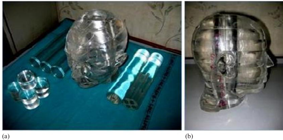
FIG. 1. A multipurpose head phantom design (a) for dosimetric purpose. The figure also shows several dosimetric inserts. Three cylinders on the right side of the phantom are for gel measurement, small discs are for film measurement, and two cylinders on the left side of phantom are for ion chamber measurements. Sagittal view (b) of the acrylic phantom.
