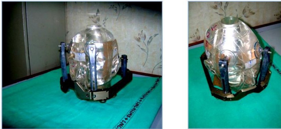
FIG. 14. The acrylic phantom fixed in Leksell stereotactic frame with carbon posts.
