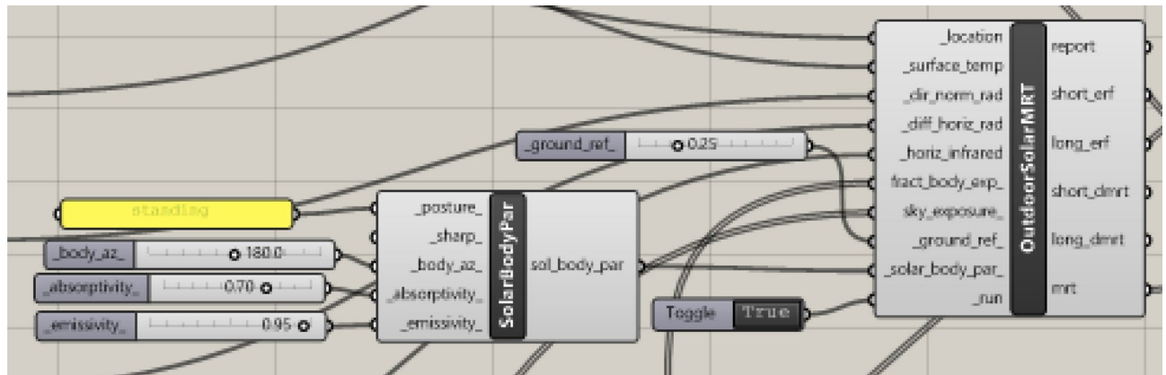
Fig. 44. Solar Body Parameters plugged in MRT component.
