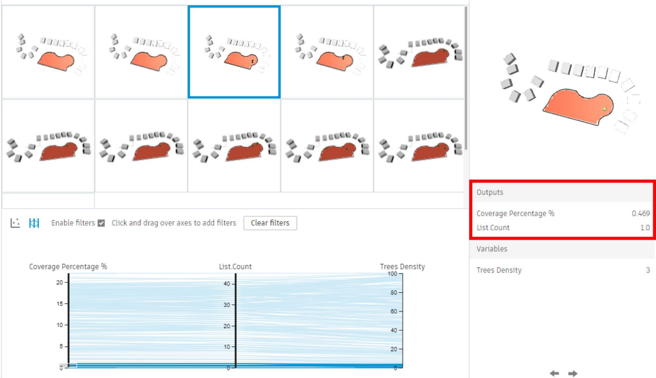
Fig. 29. Generated design solutions with the least coverage percentage 0.46%.
