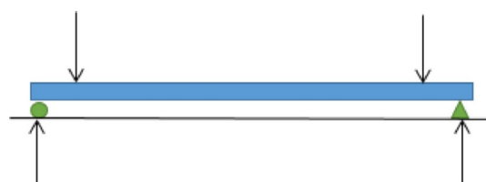
Figure 5. Bending forces operating on the rod.
