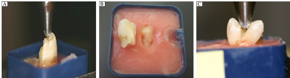
Fig. 4 Pattern of tooth fracture. A: oblique fracture. B: crown fracture at the cemento-enamel junction level. C: vertical fracture.
