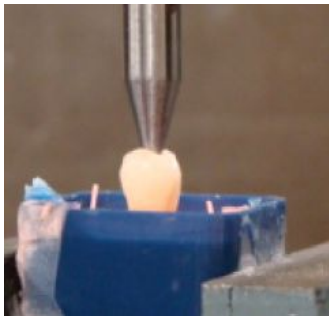
Fig. 1 Compressive strength testing of specimens carried out using a Hounsfield testing machine. The hardened steel spike with a diameter of 3 mm was positioned at the very centre of the occlusal surface of the tooth crown between buccal and palatal cusps.
