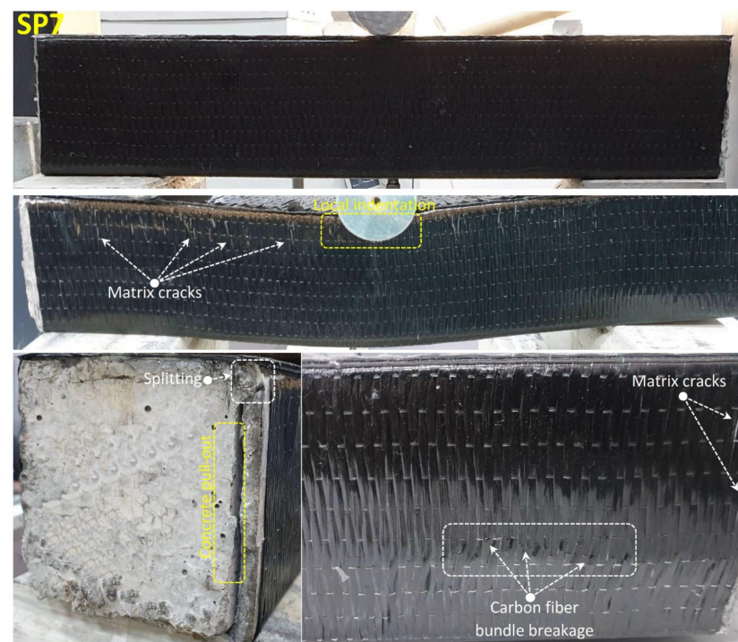
Figure 16. Undamaged and damaged specimen images of SP7.
