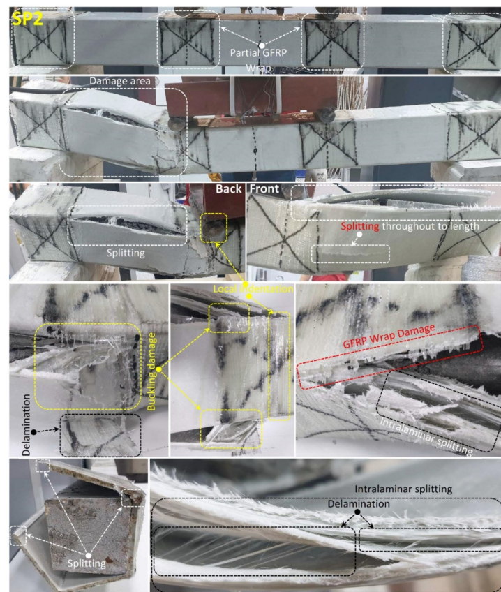
Figure 11. Undamaged and damaged specimen images of SP2.
