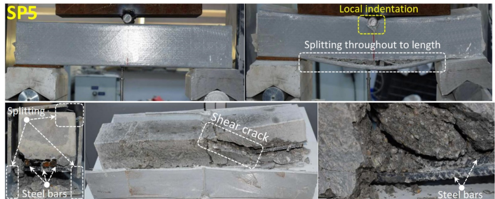
Figure 14. Undamaged and damaged specimen images of SP5.
