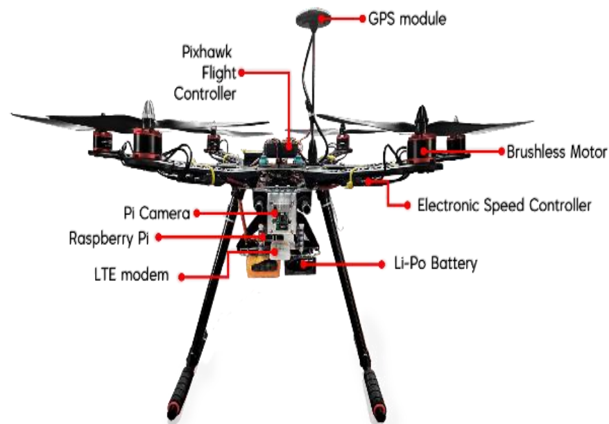
Figure 5. The developed drone prototype with an LTE-based control system.
