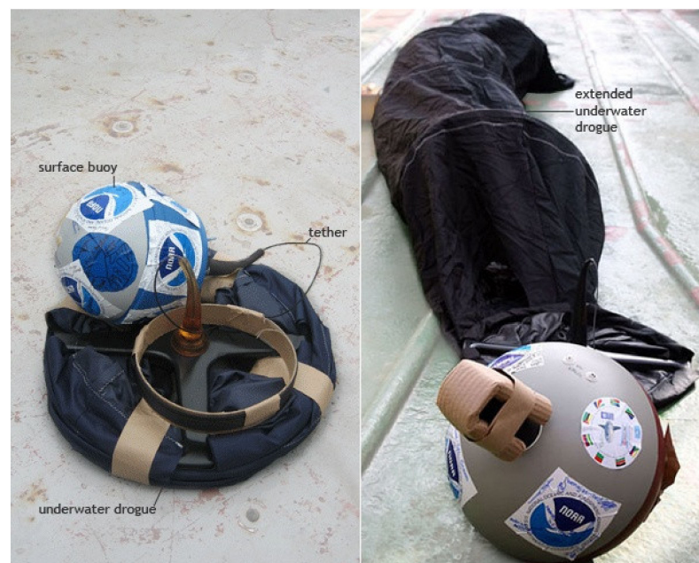
Figure 1. A drifter neatly compressed for deployment (left) and with the nylon drogue fully extended (right), as it will be in the water once the cardboard wraps dissolve. Photos courtesy of National Oceanic and Atmospheric Administration (NOAA)—Atlantic Oceanographic and Meteorological Laboratory.
