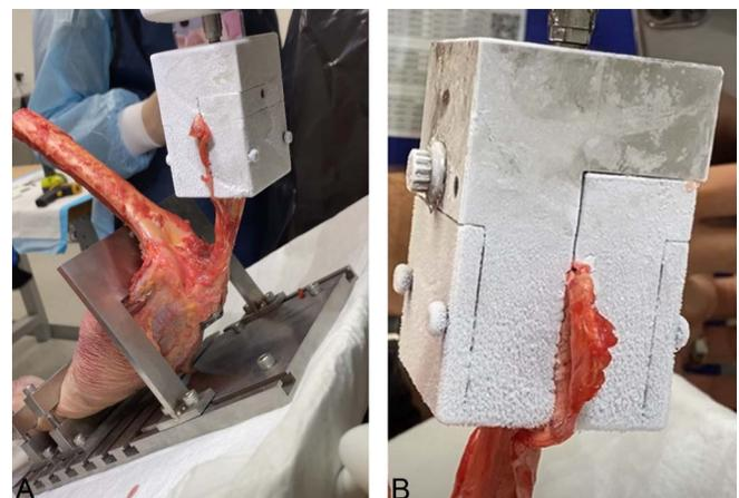
**FIGURE 2.** Custom jig used to stabilize the specimens for mechanical testing. A, The forearm is held with brackets in pronation and the elbow in flexion. The line of pull of the triceps is 60 degrees to the ulna and in line with the olecranon screws. B, A cryo-clamp was developed with dry ice-filled chambers to secure the triceps.
