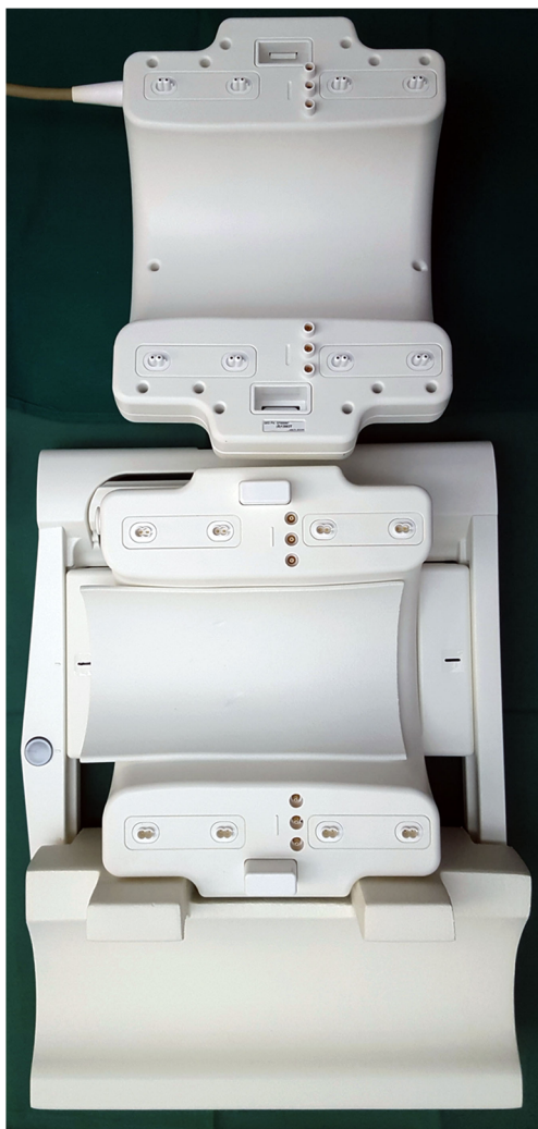
Fig. 1 Photograph of an opened, commercially available, dedicated 18-channel transmit / receive knee coil (Quality Electrodynamics, Mayfield Village, OH) for a clinical 3.0 T MR system (Siemens Healthcare, Erlangen Germany)
