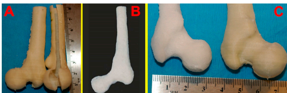
Figure 2. Two identical molds were successfully 3D printed as demonstrated in (A), one of which was sliced open to show the interior. The anatomically-shaped scaffold was also successfully generated as shown in (B) and it has the same detailed external anatomical characteristics as the mold (C).
