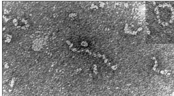
Figure 2: Electron microscopy showing molecular aggregates of mutated alpha-1 antitrypsin molecules in hepatocytes
